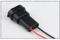
**Step 4:** Having noted the proper polarity for your car, insert the wires into the connector. Note: They must be oriented as seen in step 3.
