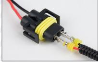
Step 3: Insert wires from the LED Bulb into your car's fog lamp connector as shown. If the lights are operational, this is the correct polarity. If not, they must be reversed.
